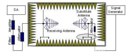
In the chamber, a substitution antenna for the frequency band of interest is placed at the reference point of the chamber. An RF Signal source for the frequency band of interest is connected to the substitution antenna with a cable that has been constructed to not interfere with the radiation pattern of the antenna. A power  $(P_{\text{Mea}})$  is applied to the input of the
