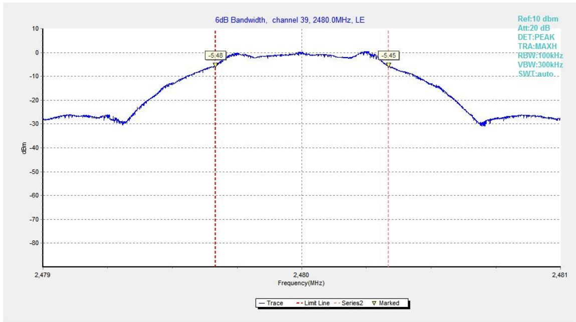
Fig.22. 6dB Bandwidth: GFSK, 2480 MHz
