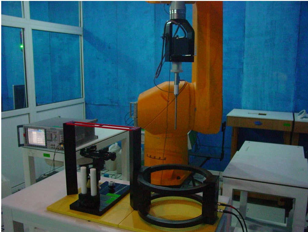
Picture A1: HAC T-Coil System Layout
