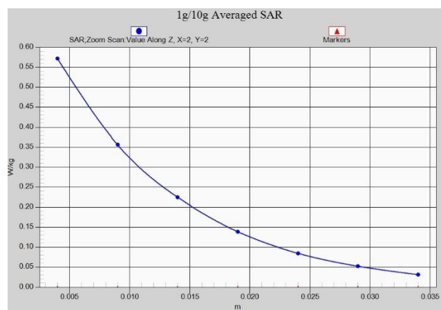
Fig. 1-5 Z-Scan at power reference point (PCS1900)
