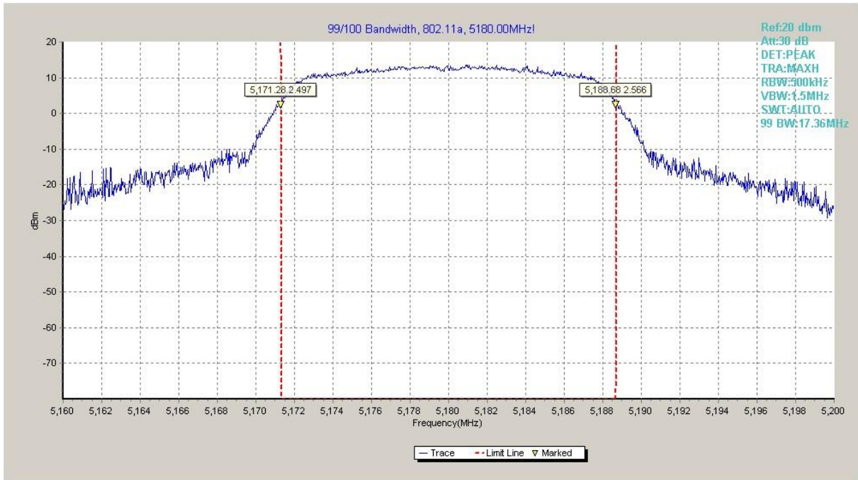
Fig.77 99% Occupied bandwidth (802.11a, 5180MHz)
