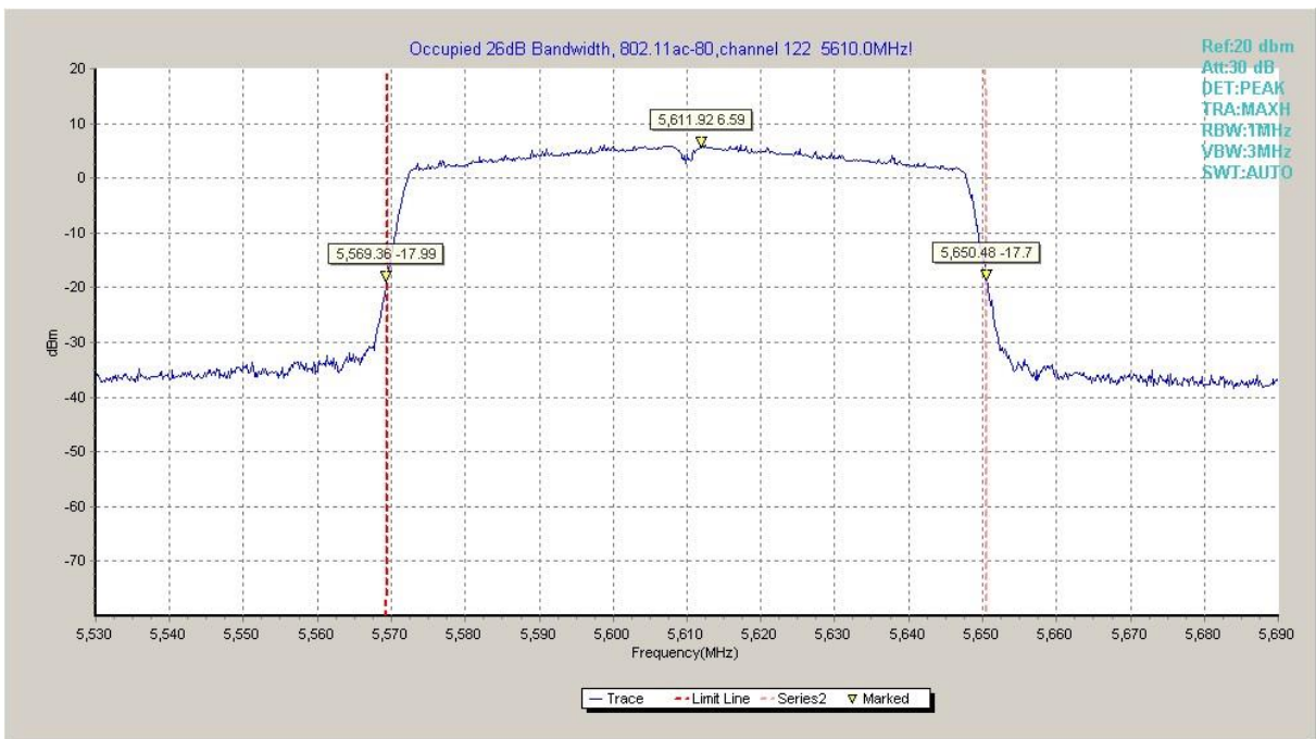
Fig.50 Occupied 26dB Bandwidth (802. 11ac-HT80, 5610MHz)
