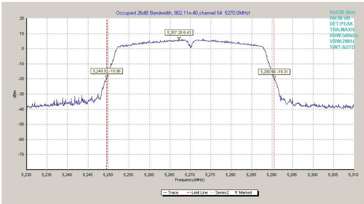
Fig.33 Occupied 26dB Bandwidth (802.11n-HT40, 5270MHz)
