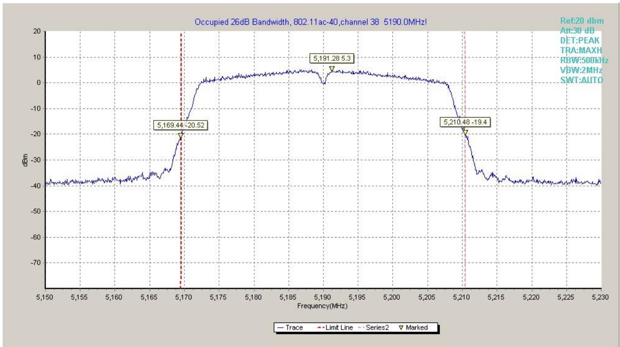
Fig.39 Occupied 26dB Bandwidth (802.11ac-HT40, 5190MHz)
