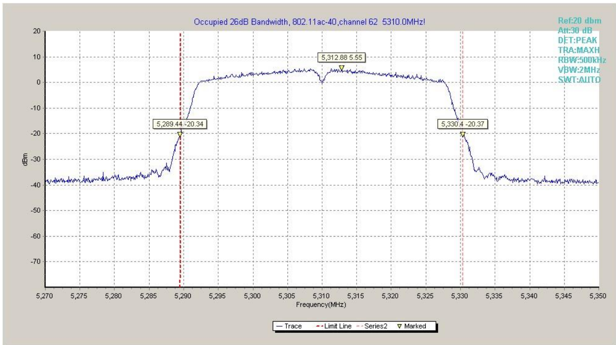
Fig.42 Occupied 26dB Bandwidth (802.11ac-HT40, 5310MHz)
