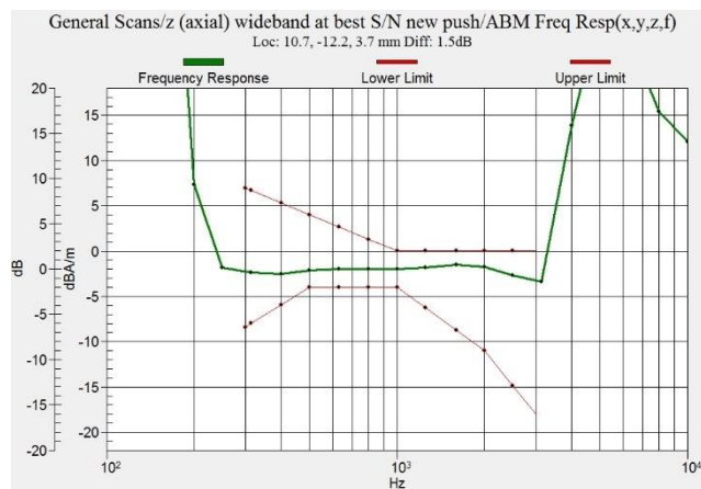
Figure C.2 Frequency Response of LTE B66
