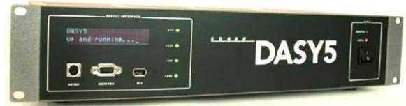
Picture C.8 Server for DASY 5
