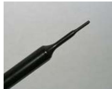
Picture C.2 Near-field Probe
