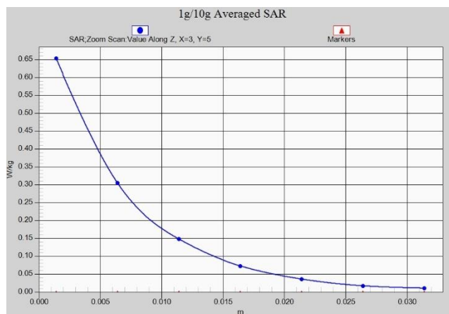
Fig. 1-27 Z-Scan at power reference point (2450 MHz)
