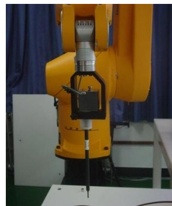
Picture C.2 Near-field Probe
