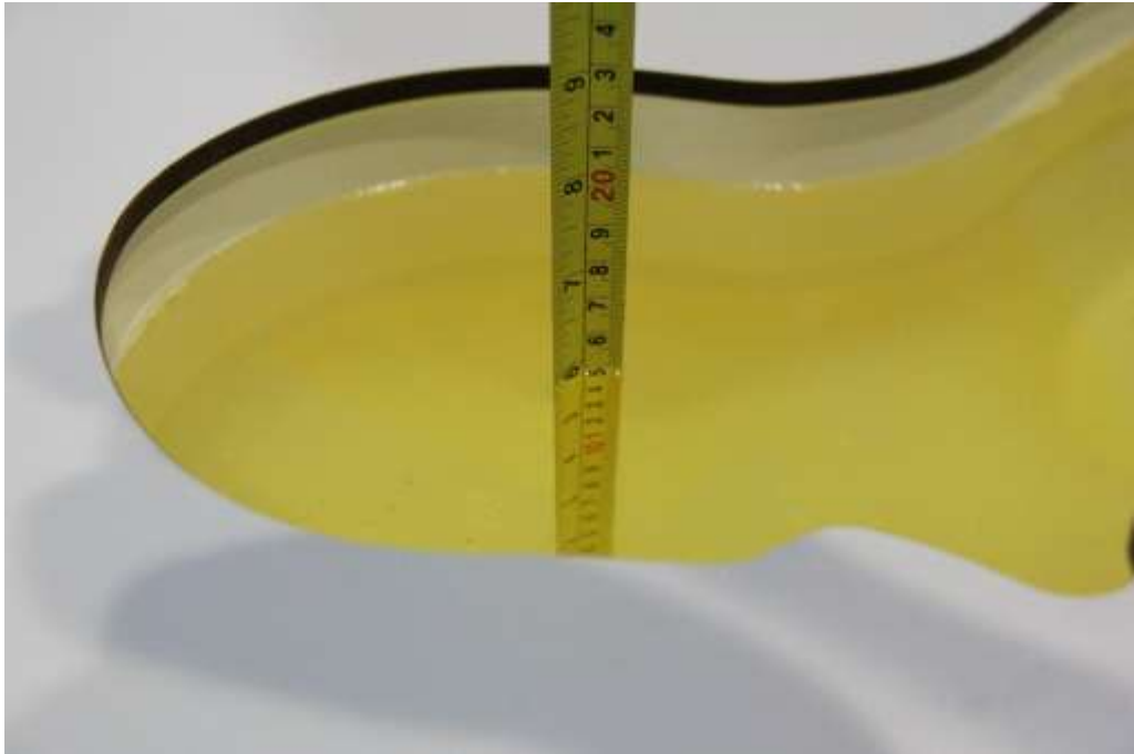
Picture 7-4: Liquid depth in the Head Phantom(2300MHz)
