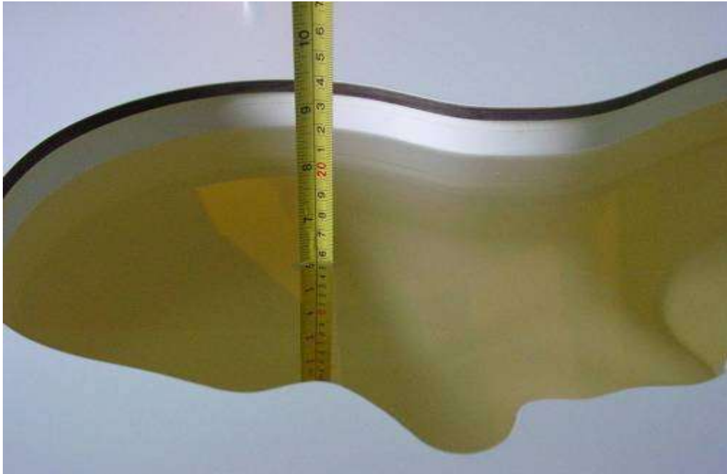
Picture 15-1: Liquid depth in the Head Phantom (750MHz)
