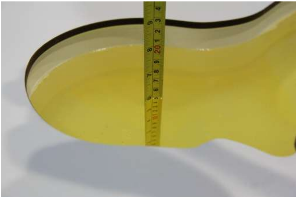
Picture 7-5: Liquid depth in the Head Phantom(2450MHz)
