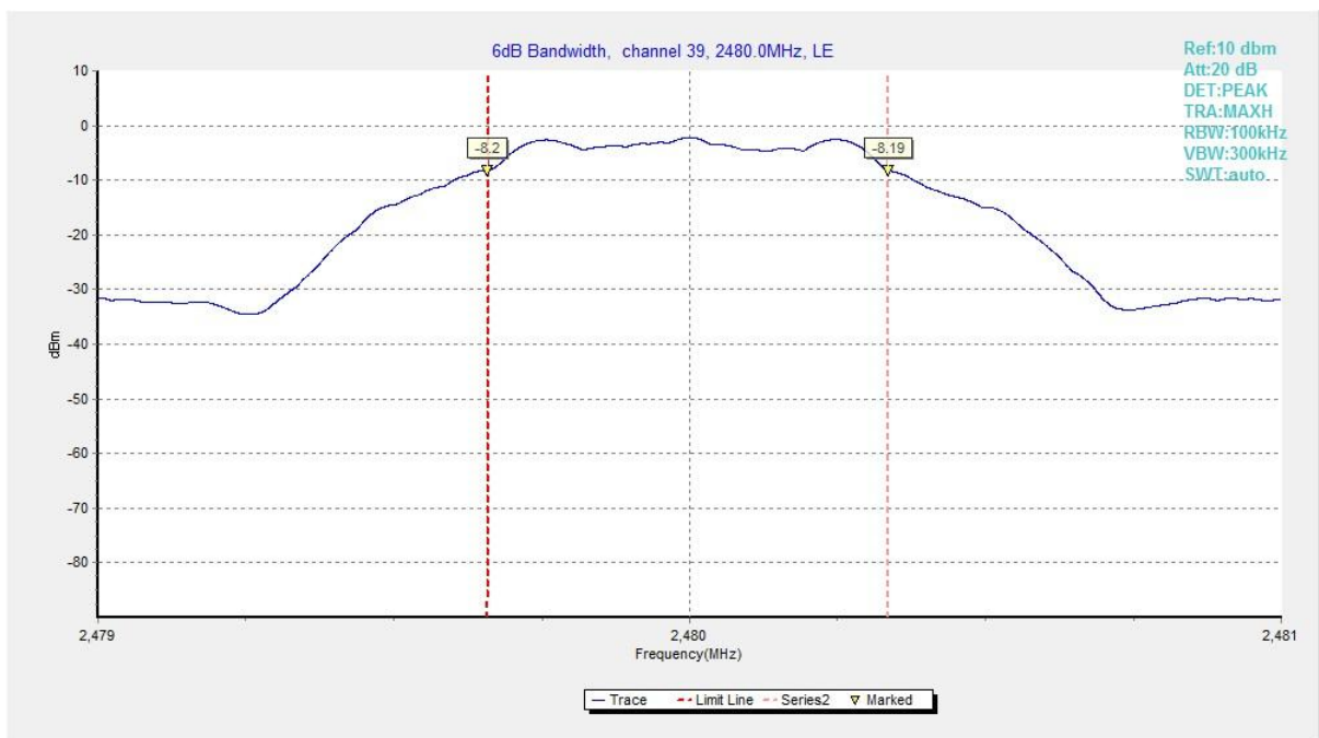
Fig.6 6dB Bandwidth (Ch 39), LE 1M
