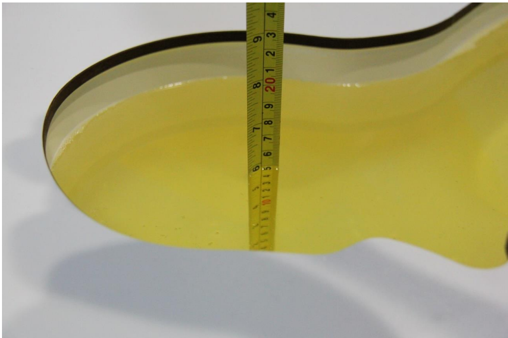
Picture 7-5: Liquid depth in the Head Phantom(2450MHz)
