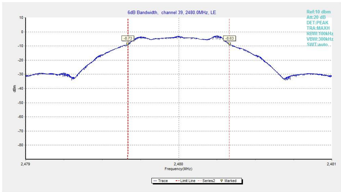
Fig.22. 6dB Bandwidth: GFSK, 2480 MHz
