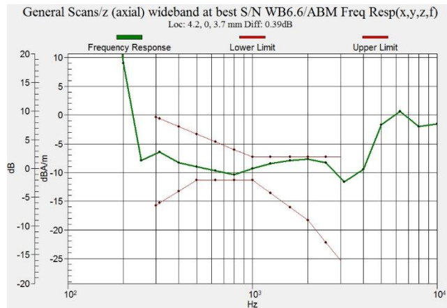
Figure C.2 Frequency Response of LTE B25
