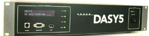
Picture C.8 Server for DASY 5
