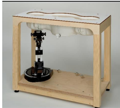
Picture C.10: SAM Twin Phantom
