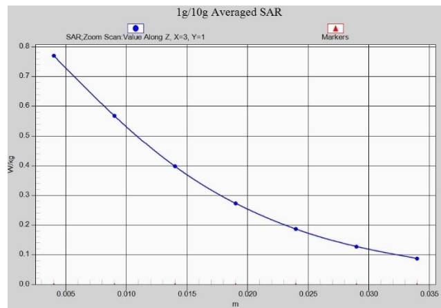
Fig. 1-31 Z-Scan at power reference point (LTEB26)
