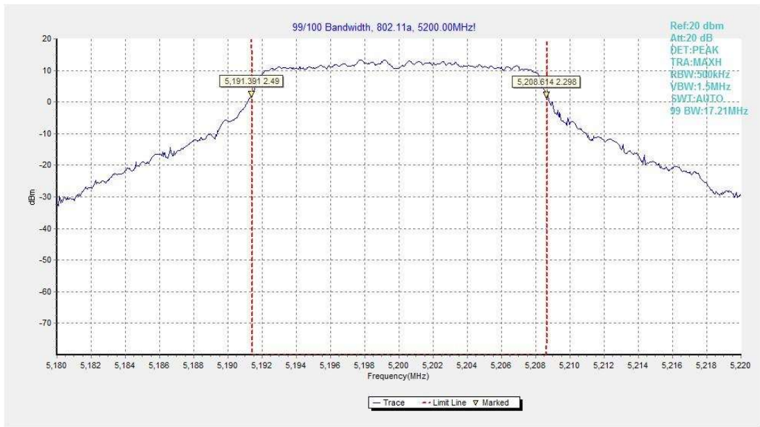
Fig.77 99% Occupied bandwidth (802.11a, 5200MHz)
