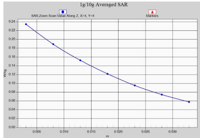
Fig. 1-16 Z-Scan at power reference point (LTE Band 5)
