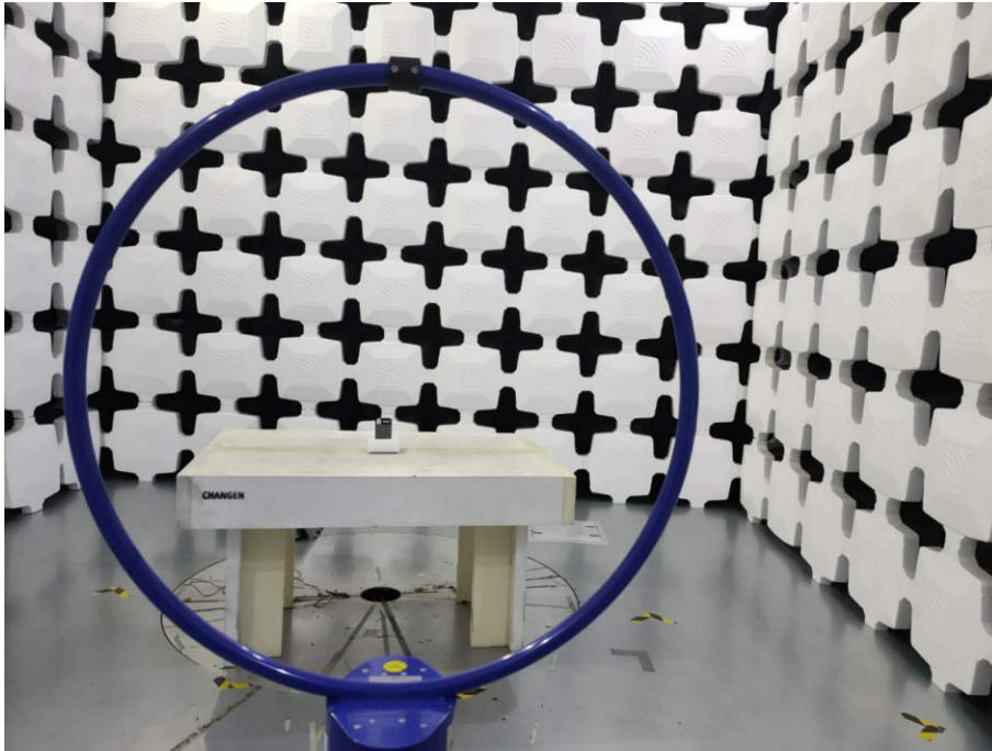
1. Radiated Emissions (Part 15C) (9kHz-30MHz)
