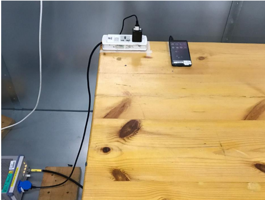
5. Conducted Emission (Part 15C, Charging Mode)
