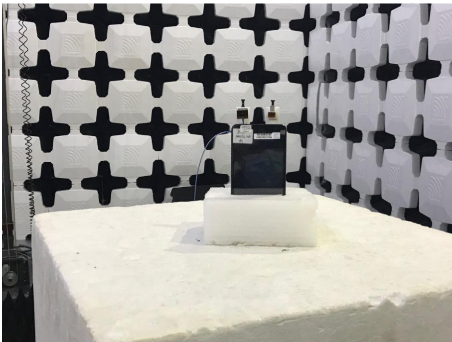
4. Radiated Emissions (Part 15C) (18-26.5GHz)
