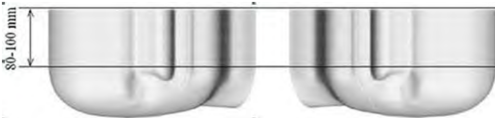
F-4. Sagittally bisected phantom with extended perimeter (shown placed on its side as used for SAR measurements)
