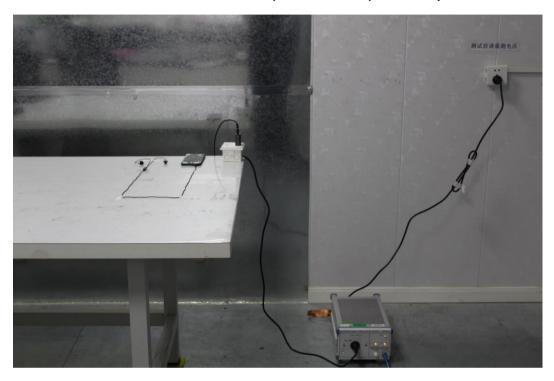
**Radiated Emissions Test Setup**
