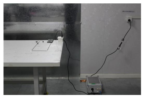
**Radiated Emissions Test Setup**
