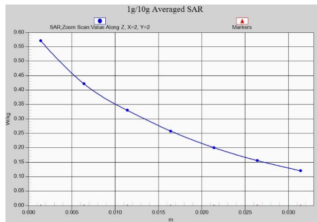
Fig. 1-12 Z-Scan at power reference point (WCDMA850)
