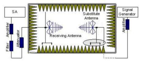
In the chamber, a substitution antenna for the frequency band of interest is placed at the ©Copyright. All rights reserved by CTTL. Page 14 of 55
