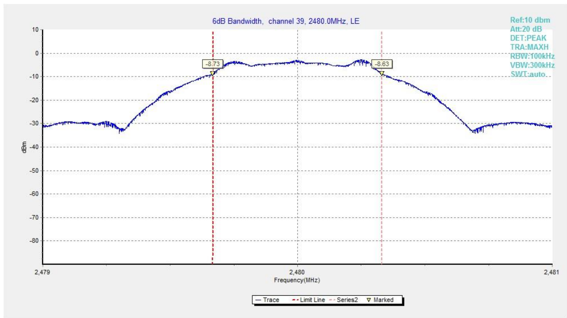
Fig.22. 6dB Bandwidth: GFSK, 2480 MHz
