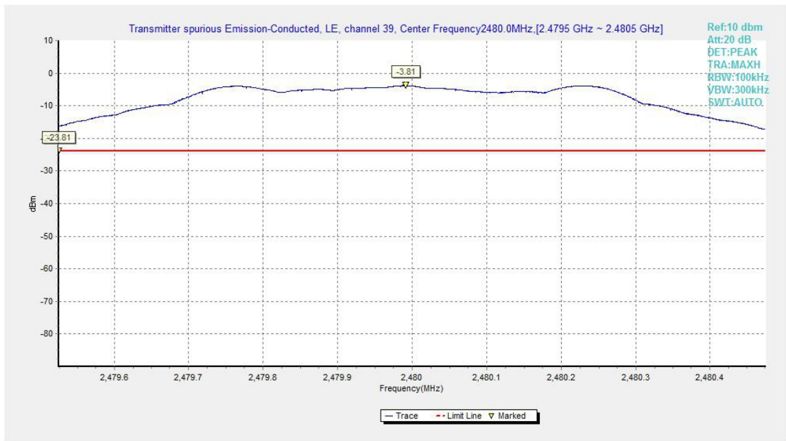
Fig.13. Transmitter Spurious Emission - Conducted: GFSK, 2480 MHz
