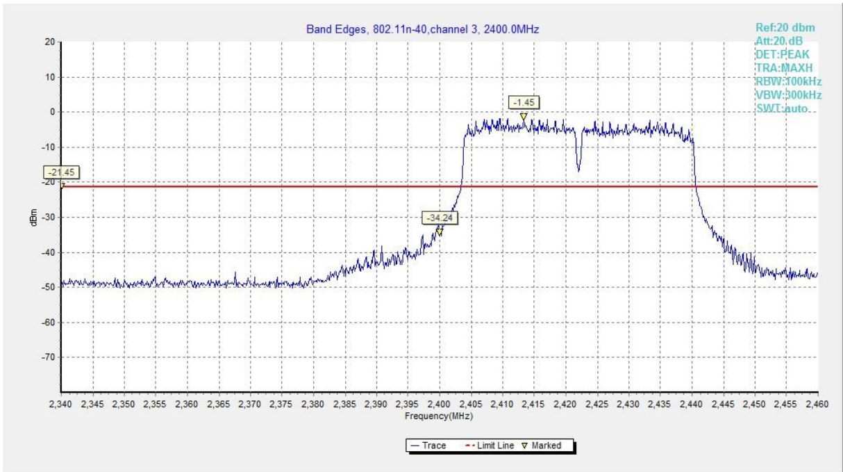
Fig.A.5.7 Band Edges (802.11n-HT40, Ch 3)
