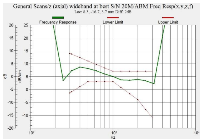
Figure C.6 Frequency Response of LTE B2
