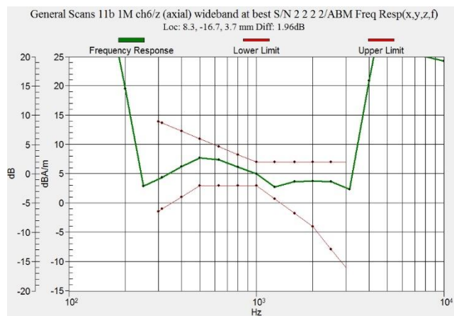
Figure C.12 Frequency Response of WiFi-2.4G
