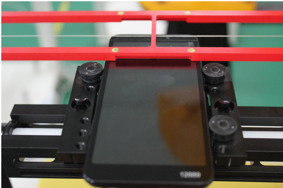
Picture 2: EUT Positioning for RF/T-coil
