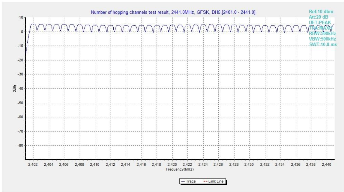
Fig.94. Number of hopping frequencies: GFSK, Channel 0 - 39
