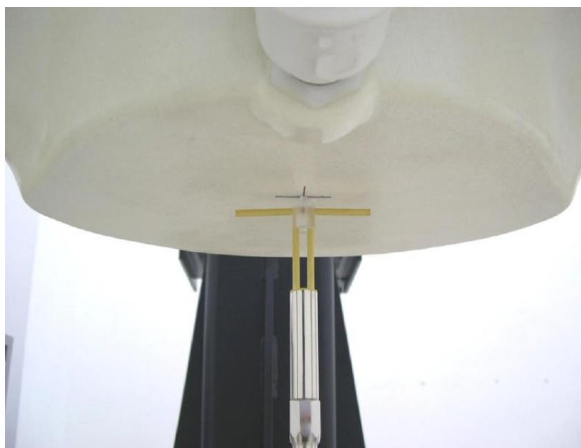
Picture 8.2 Photo of Dipole Setup
