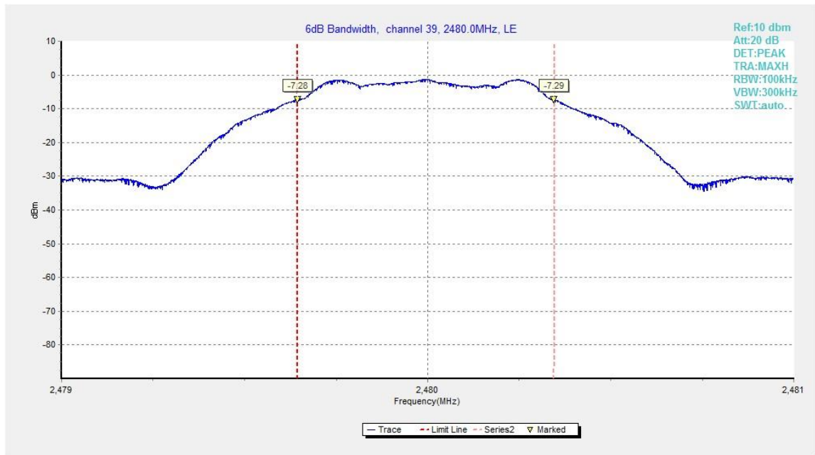
Fig.22. 6dB Bandwidth: GFSK, 2480 MHz
