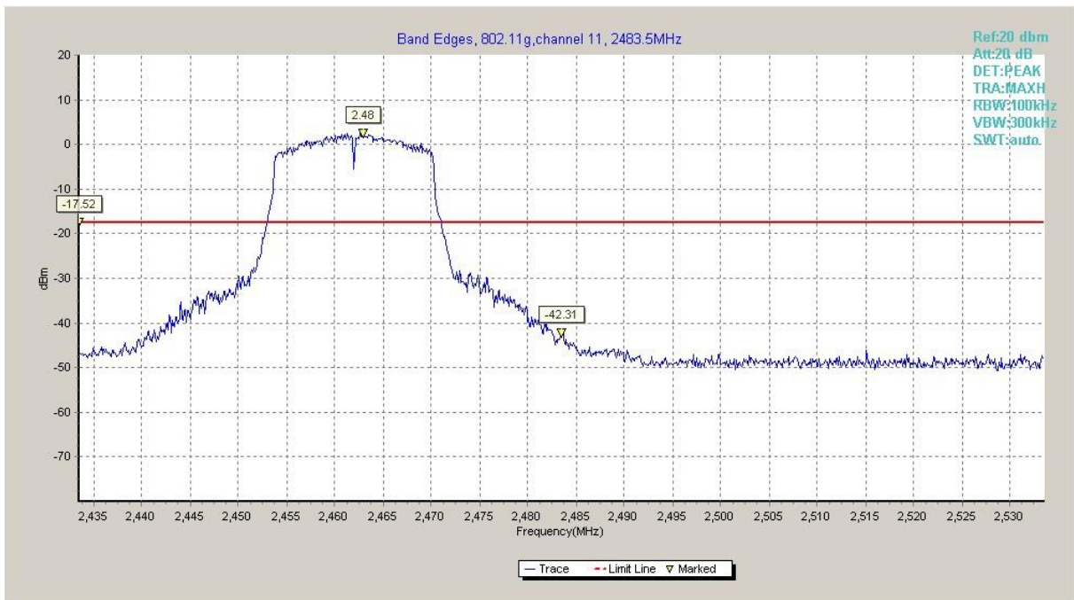
Fig.A.5.4 Band Edges (802.11g, Ch 11)
