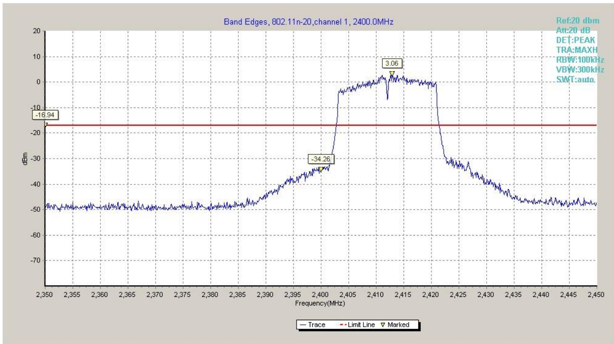
Fig.A.5.5 Band Edges (802.11n-HT20, Ch 1)
