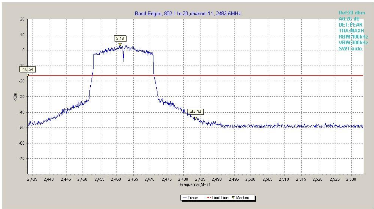
Fig.A.5.6 Band Edges (802.11n-HT20, Ch 11)
