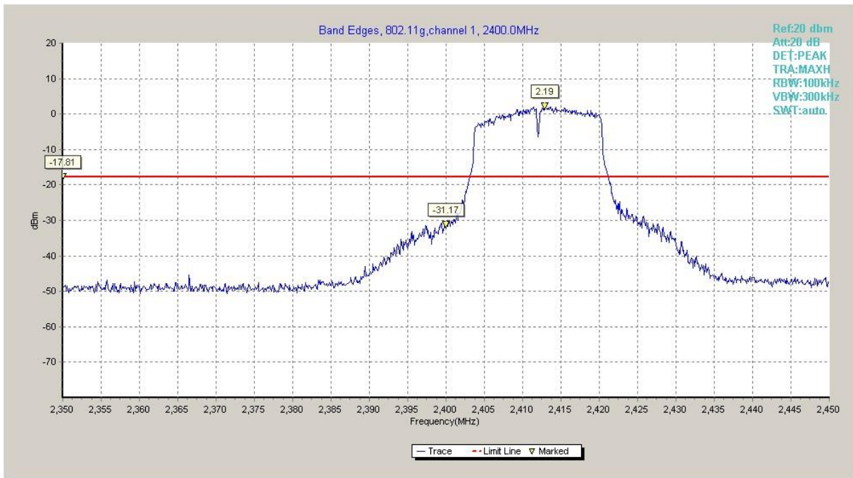
Fig.A.5.3 Band Edges (802.11g, Ch 1)
