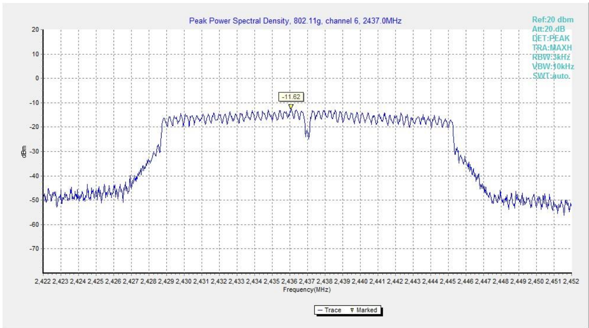
Fig.A.3.5 Power Spectral Density (802.11g, Ch 6)
