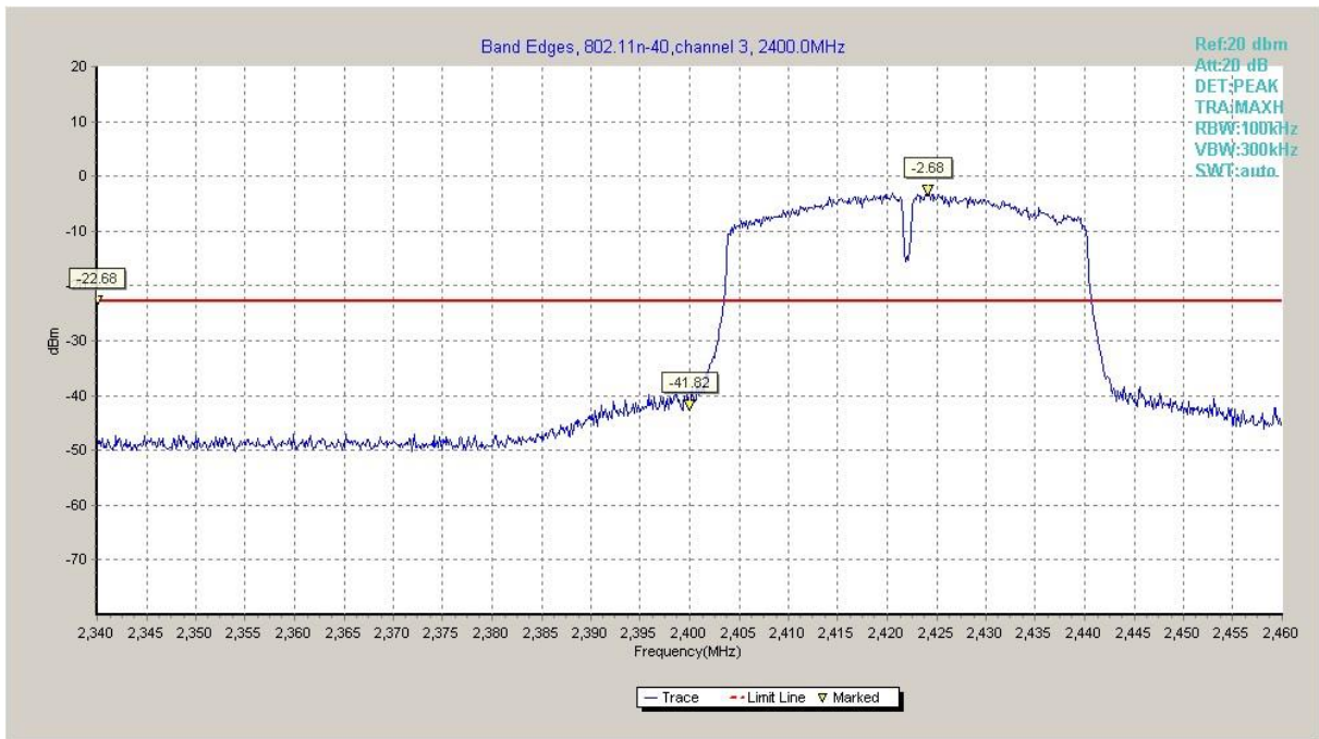
Fig.A.5.7 Band Edges (802.11n-HT40, Ch 3)
