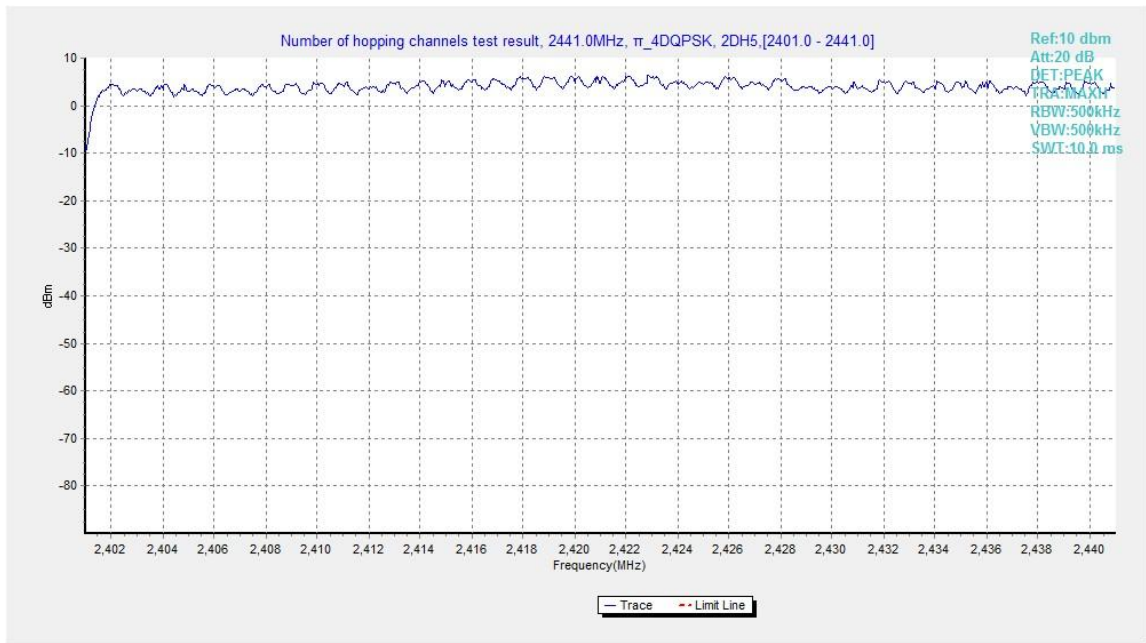
Fig.96. Number of hopping frequencies: \pi/4 DQPSK, Channel 0 - 39
