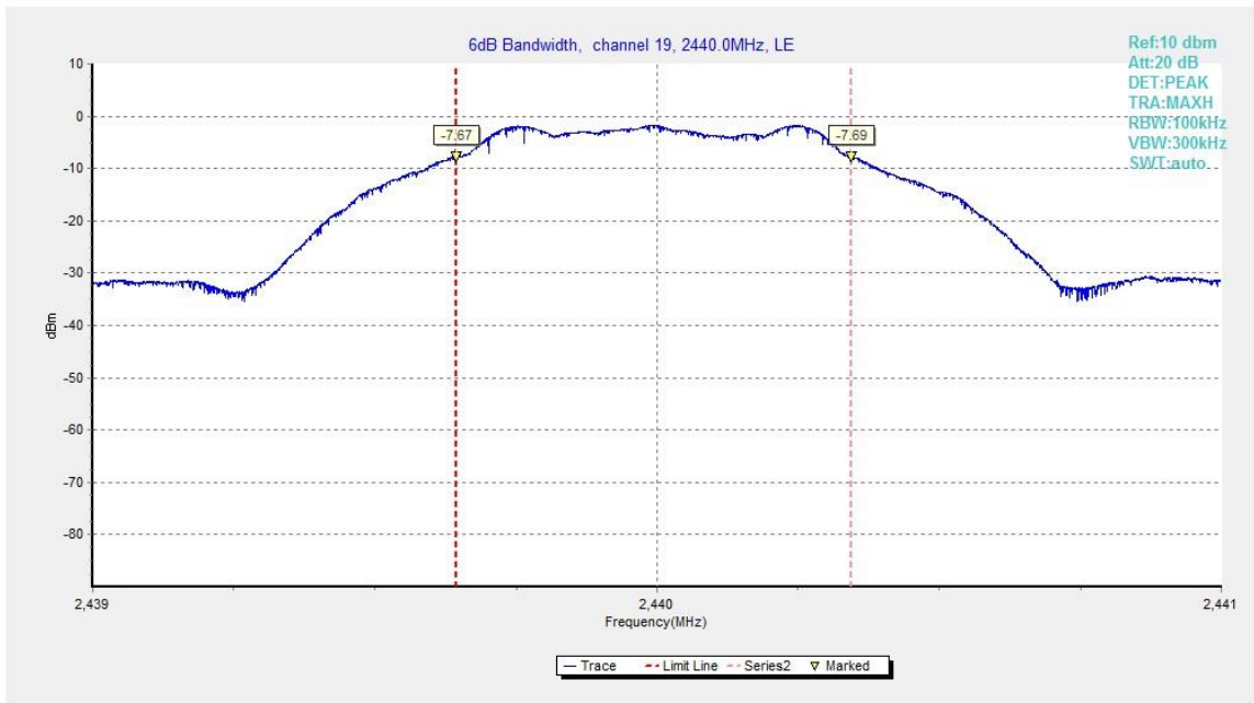
Fig.21. 6dB Bandwidth: GFSK, 2440 MHz
