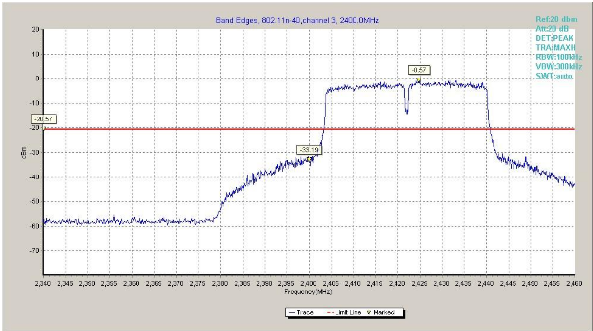
Fig.A.5.7 Band Edges (802.11n-HT40, Ch 3)
