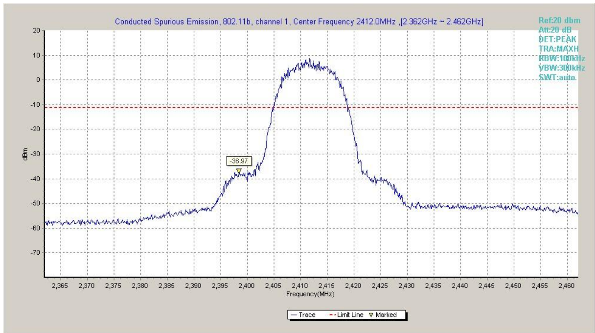
Fig.A.6.1.1 Transmitter Spurious Emission - Conducted (802.11b, Ch1, Center Frequency)
