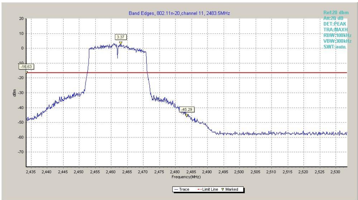
Fig.A.5.6 Band Edges (802.11n-HT20, Ch 11)
