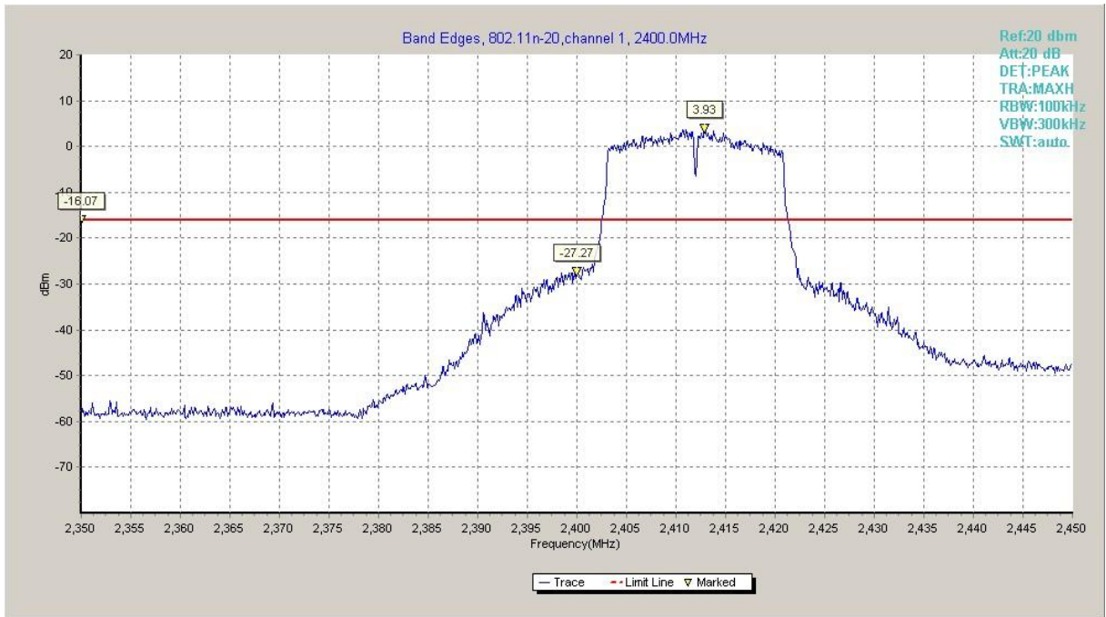
Fig.A.5.5 Band Edges (802.11n-HT20, Ch 1)
