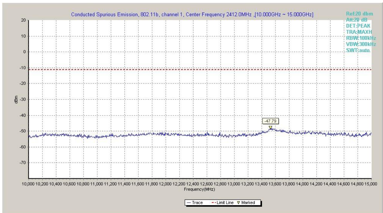
Fig.A.6.1.6 Transmitter Spurious Emission - Conducted (802.11b, Ch1, 10 GHz-15 GHz)
