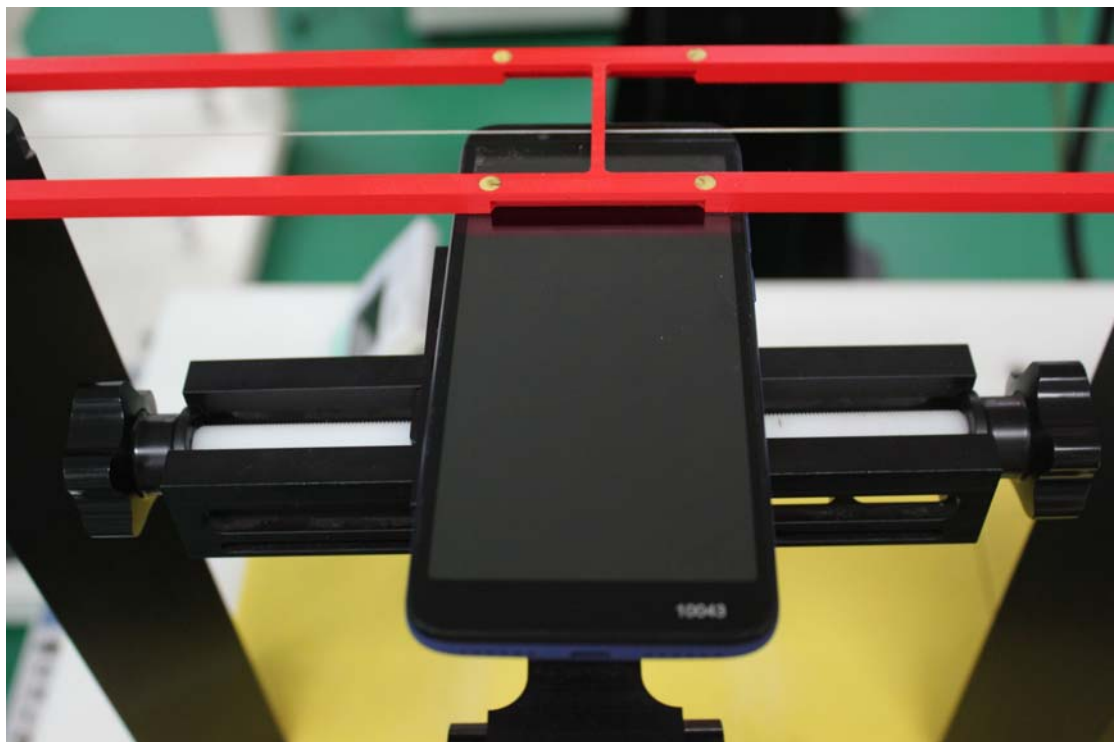
Picture 2: EUT Positioning for RF/T-coil
