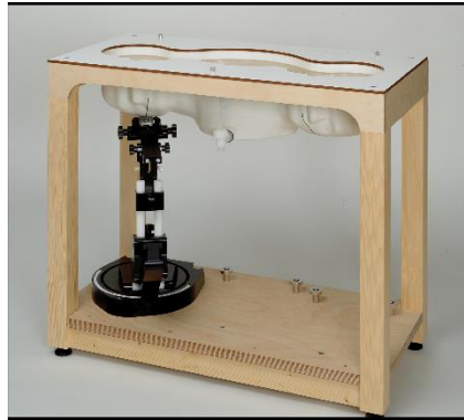
Picture C.10: SAM Twin Phantom
