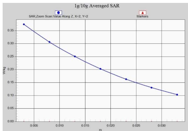
Fig.A.1- 20 Z-Scan at power reference point (LTE band14)
