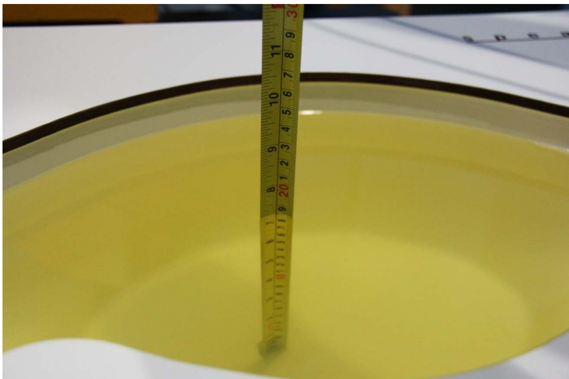
Picture 7-8 Liquid depth in the Flat Phantom (1900MHz)
