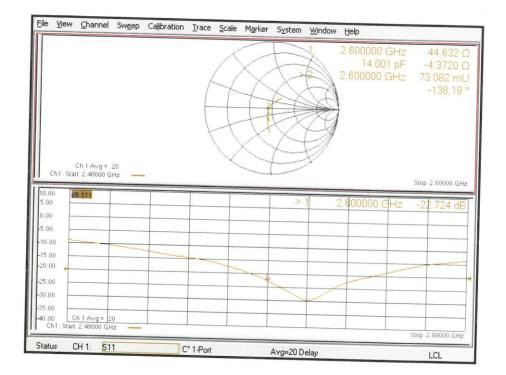
Impedance Measurement Plot for Body TSL
