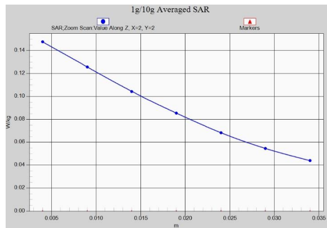
Fig.A.1- 15 Z-Scan at power reference point (LTE Band5)
