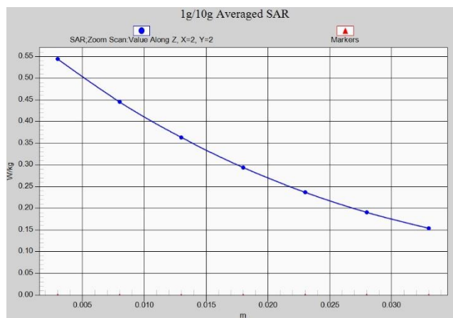
Fig.A.1- 20 Z-Scan at power reference point (LTE Band12)
