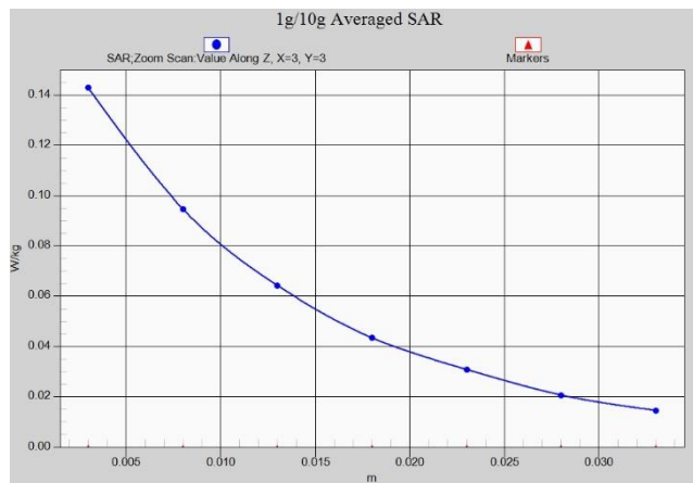
Fig.A.1- 9 Z-Scan at power reference point (W1900)
