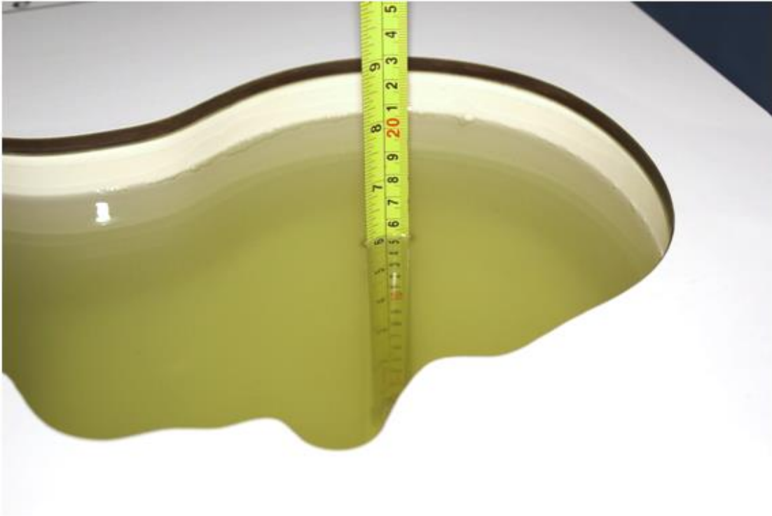
Picture 7-11 Liquid depth in the Head Phantom (2600 MHz Head)
