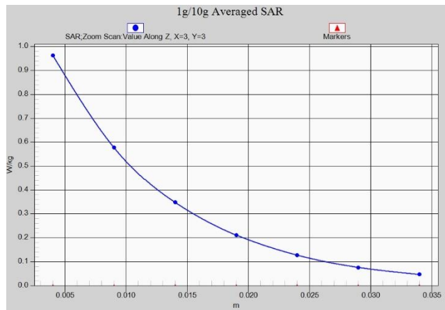
Fig.A.1- 10 Z-Scan at power reference point (W1900)
