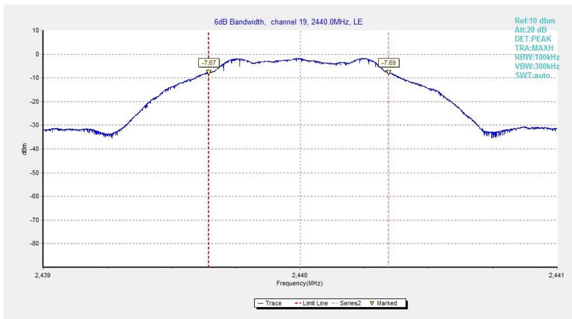
Fig.21. 6dB Bandwidth: GFSK, 2440 MHz
