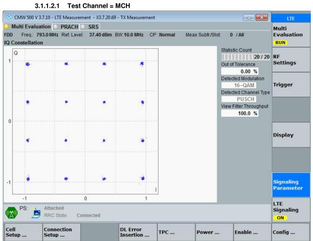
3.1.1.2 Test Mode = LTE /TM2 10MHz
