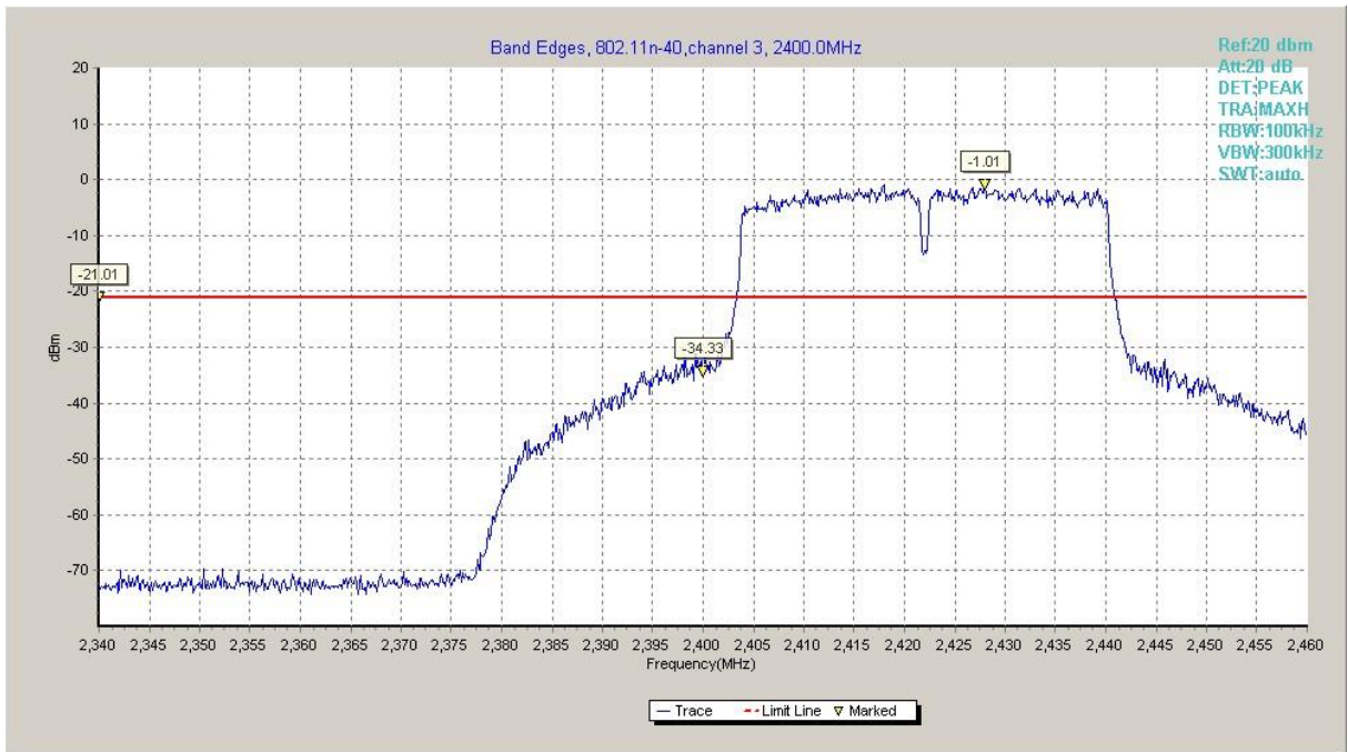
Fig.A.5.7 Band Edges (802.11n-HT40, Ch 3)
