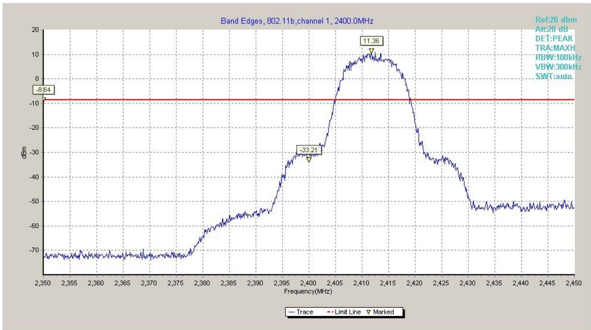
Fig.A.5.1 Band Edges (802.11b, Ch 1)
