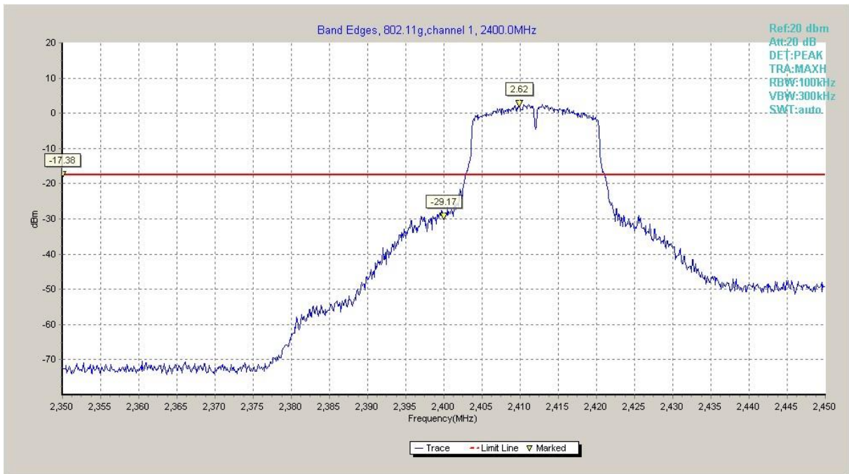
Fig.A.5.3 Band Edges (802.11g, Ch 1)
