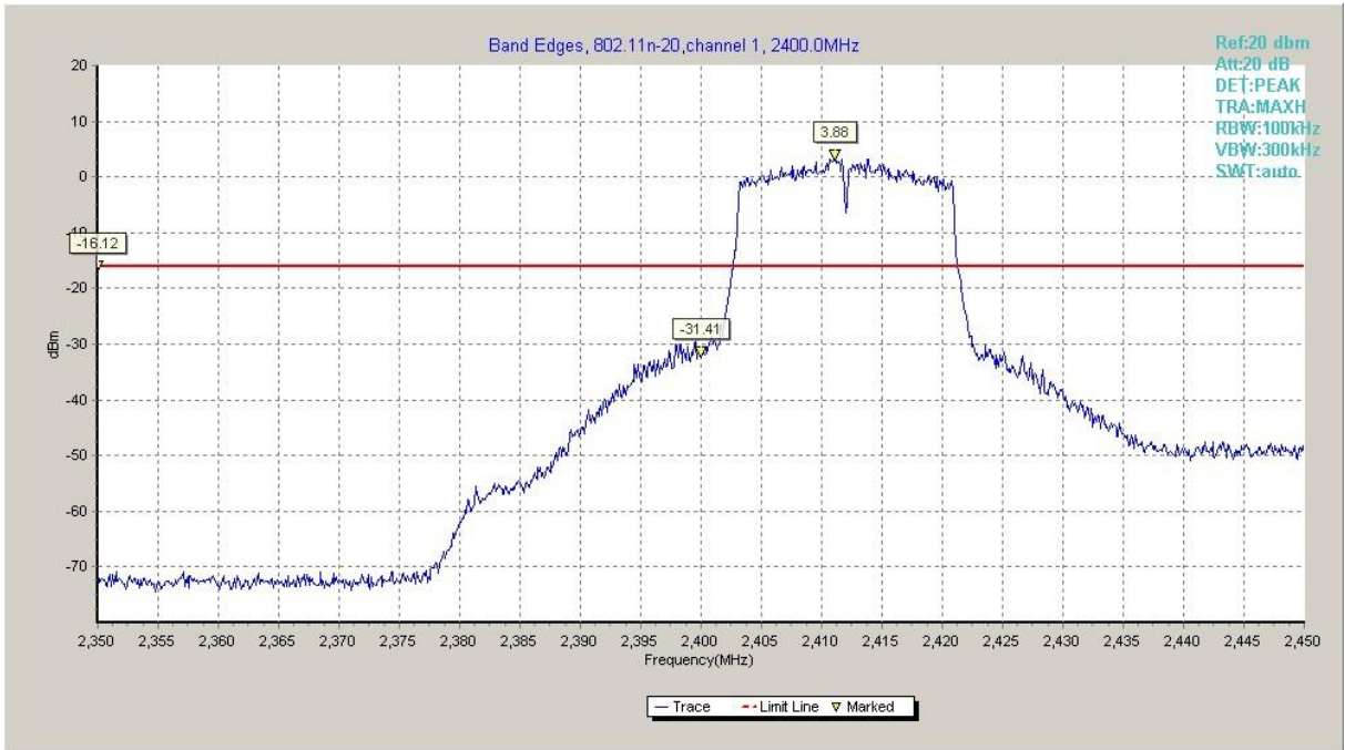
Fig.A.5.5 Band Edges (802.11n-HT20, Ch 1)
