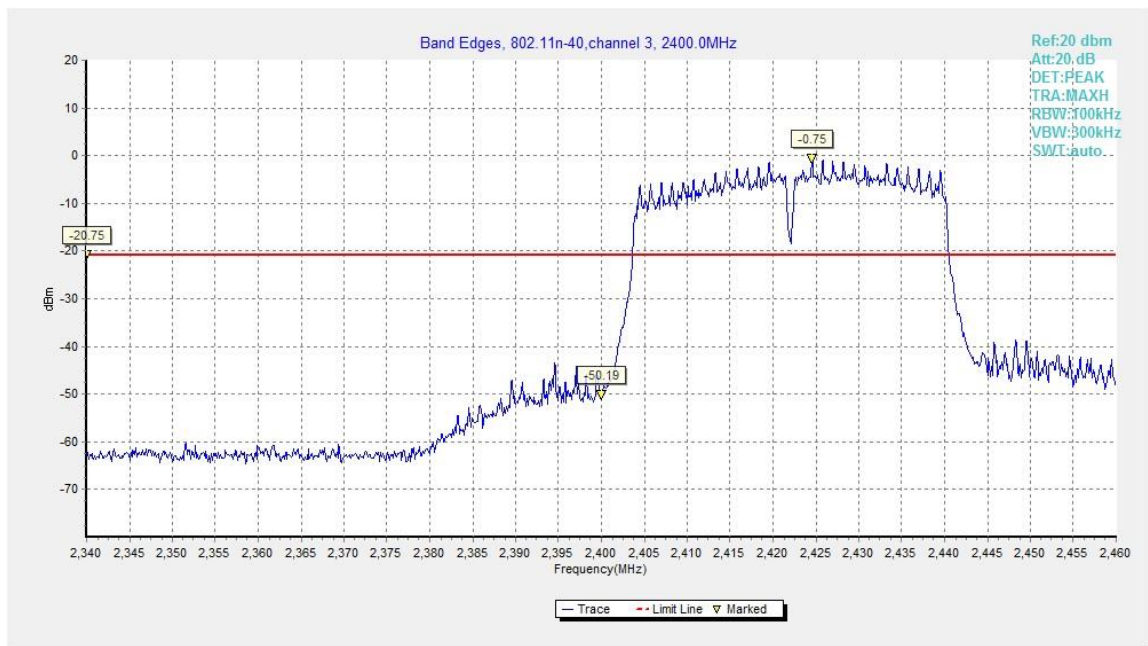
Fig.A.5.7 Band Edges (802.11n-HT40, Ch 3)
