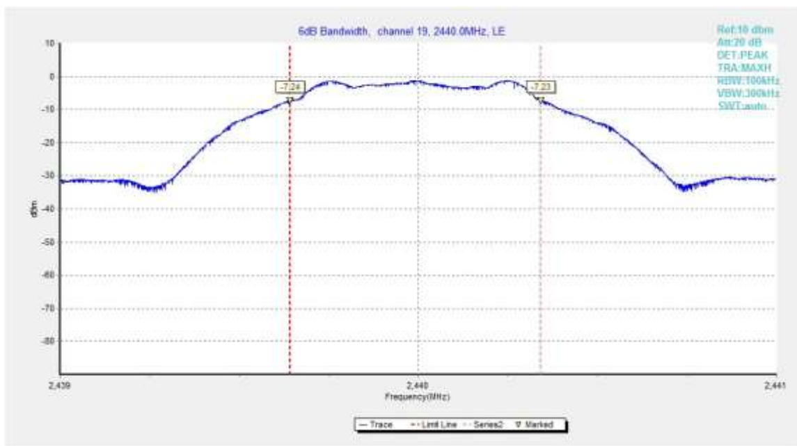
Fig.21. 6dB Bandwidth: GFSK, 2440 MHz
