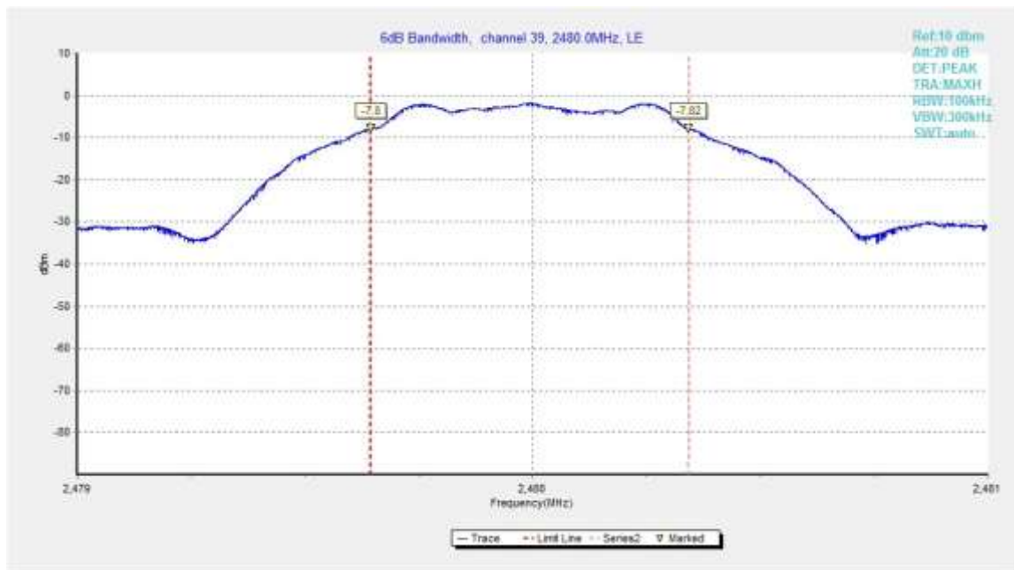
Fig.22. 6dB Bandwidth: GFSK, 2480 MHz
