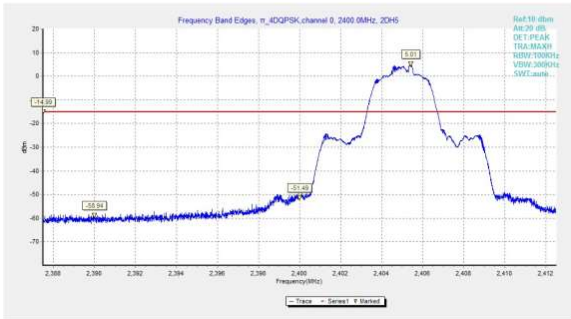
Fig.5. Frequency Band Edges: \pi/4 DQPSK, Channel 0, Hopping Off
