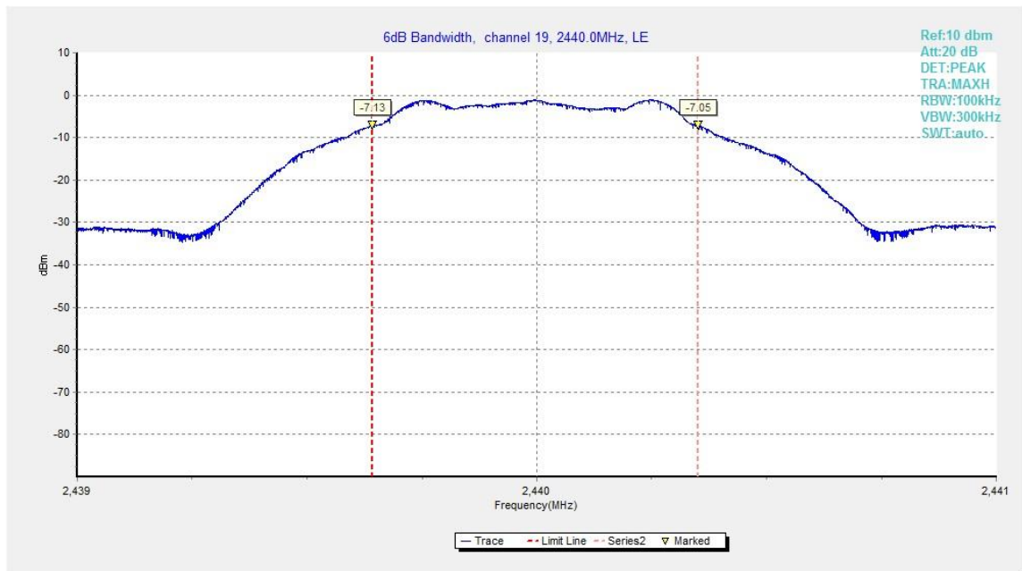
Fig.21. 6dB Bandwidth: GFSK, 2440 MHz
