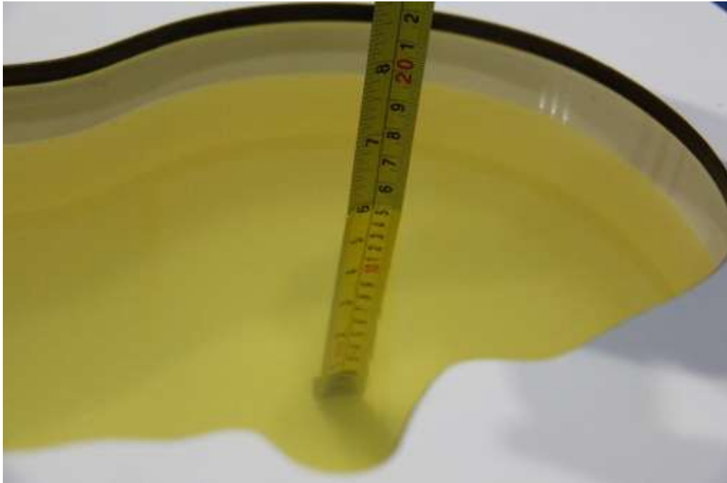
Picture 7-3: Liquid depth in the Head Phantom (1900MHz)
