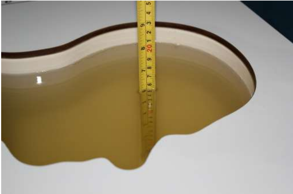
Picture 7-5: Liquid depth in the Head Phantom(2550MHz)
