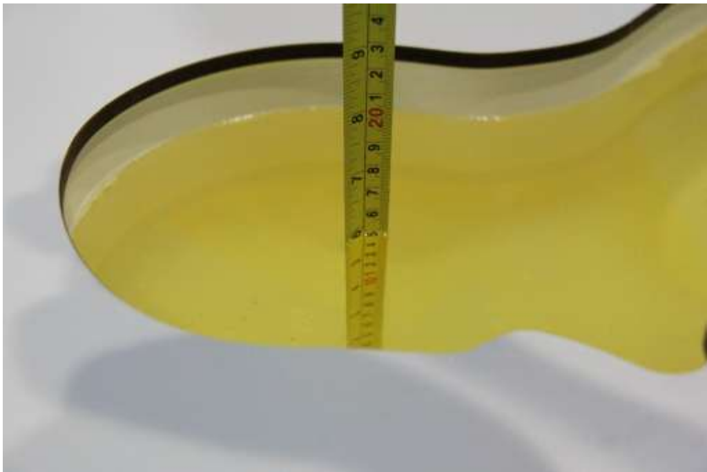
Picture 7-4: Liquid depth in the Head Phantom(2450MHz)
