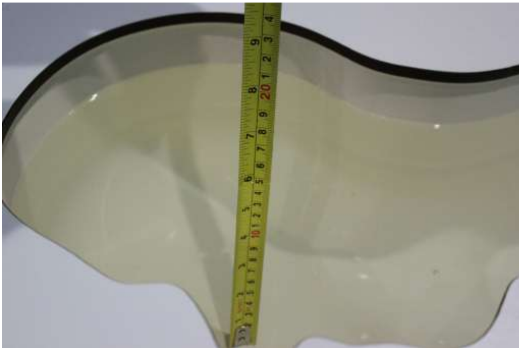
Picture 7-6: Liquid depth in the Head Phantom(5GHz)
