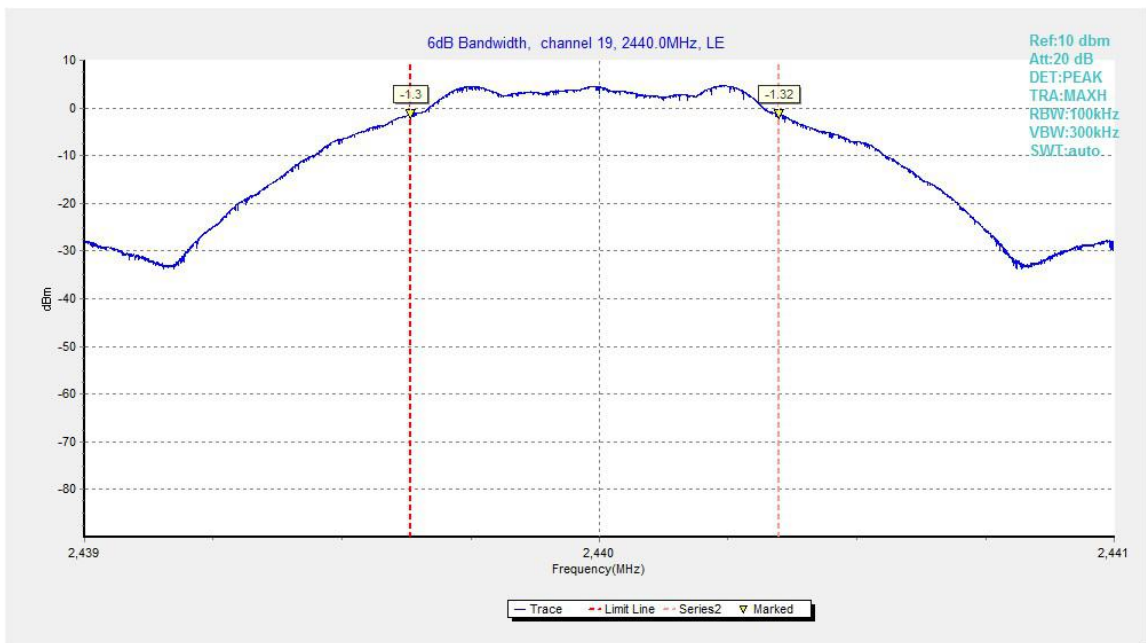
Fig.21. 6dB Bandwidth: GFSK, 2440 MHz
